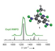
**Proof positive**: Infrared multiphoton dissociation (IRMPD) spectroscopy, with the tunable IR radiation of a free-electron laser source, provides positive identification of alkoxide adducts of 1,3,5-trinitrobenzene as prototypical anionic  $\sigma$  complexes in the gas phase (see calculated IR spectrum of 1 under the experimental IRMPD spectrum; N blue, O green, C gray, H light gray).
